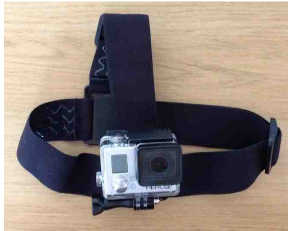
Figure 1: GoPro Hero3+ BLACK edition with head strap (Image source: Author's own photograph)
