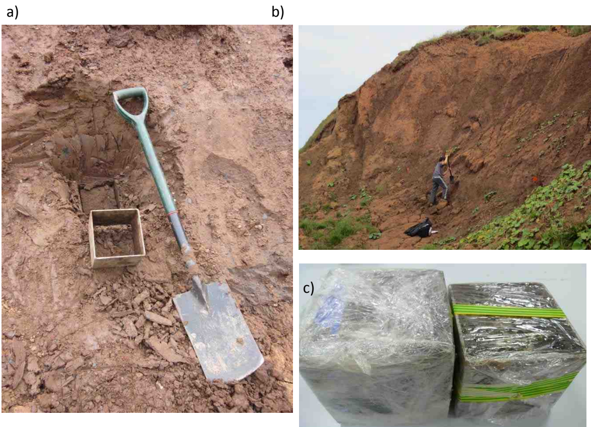
Figure 3.15 Collection of undisturbed glacial till samples at the Upper section of the cliff: a) Sampling equipment: b) Sampling location and c) Examples of undisturbed samples with cling film wrap
