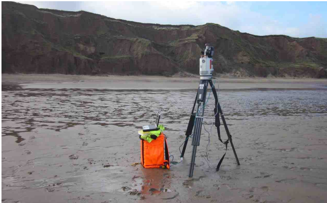
Figure 3.5 Photographs of two devices: a) Trimble GS200 device includes a tripod, a laser scanner, a generator and a computer; b) RIEGL VZ 1000 consists of a tripod, a laser scanner and a computer
