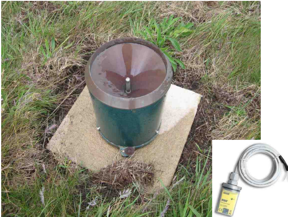
Figure 3.14 A tipping bucket rain gauge and its data logger on top of the cliff
