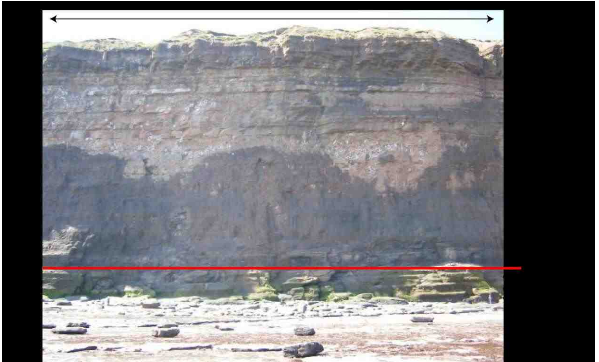
Figure 7.1: The monitored cliff section. The red line marks the upper limit of the inundation zone. 1 = cliff toe (1.6 mOD), 2 = max tide height (1.67 m above cliff toe), 3 = combined max tide, wave and set-up height (2.9 m above cliff toe). The cause of the water mark on the face is uncertain, but it does not represent inundation by the sea. This lower section of the cliff protrudes beyond the upper section and so the water mark may reflect where water has washed over the cliff top, or groundwater seepage.
