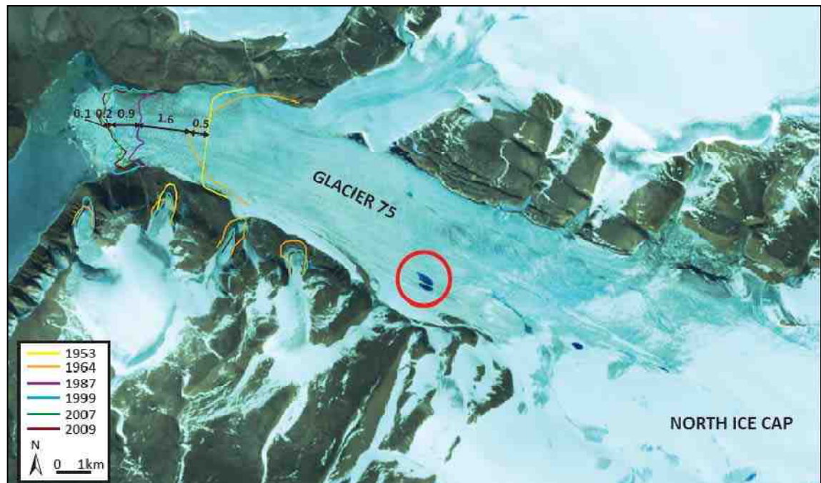
Figure 3.8: Terminus position of possible surge type Glacier 75 (Berlingske Brae) in the northwest study area mapped at six time steps between 1953 and 2009. The red circle highlights a surface meltwater pond. Underlying image is the 1999 Landsat TM base image, displayed as band 4,3,2 (red, green, blue) combination.
