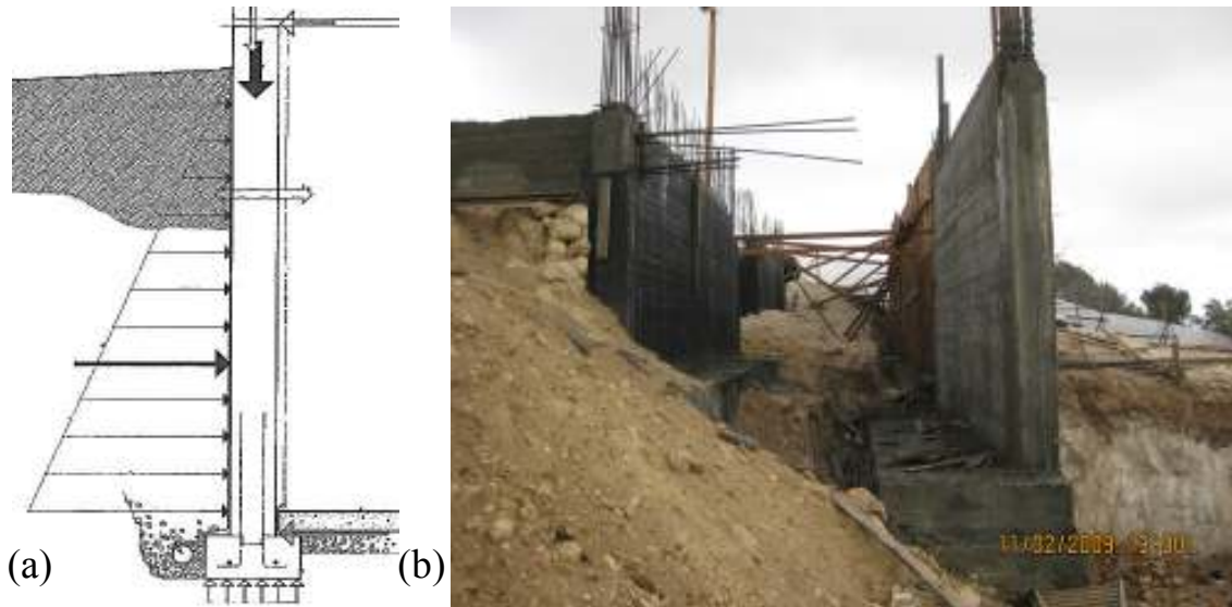
Figure (16): (a) A section in a Foundation Wall, (b) Photo of a foundation wall in a project in the West Bank
