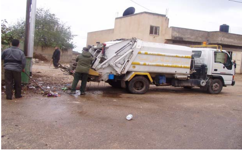
Figure (3.4): Three tons solid waste compactor
