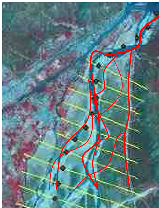
Fig 3.4: Visual description of the braiding index method. The image above has been cropped from the IRS image. The yellow lines show the width of the channel over which braids were counted. This was a crude method of counting how many channels of water (blue) crossed any one yellow line. The brown dots identify the points where width of channel belt was measured and therefore it to be consistent with channel counting, the same points of measurement were used.
