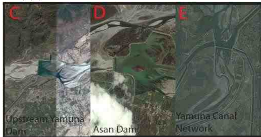
Fig 1.3b. The three satellite images above illustrate the three main river diversions on the Yamuna within the study reach. The red letters correspond to the red letters on Fig 1.2. C is located upstream (west) of Vikasnagar, D is located immediately upstream of Paonta Sahib, and E shows the Eastern and Western Yamuna Canal Network. The satellite image is from Google maps.
