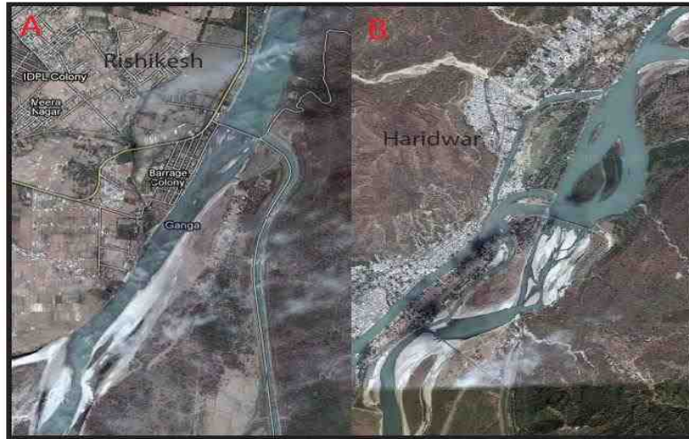
Fig 1.3a. The two satellite images above illustrate the two main river diversions on the Ganges within the study reach. The red letters correspond to the letters on Fig 1.2 above. A is located at Rishikesh, and B, the more significant river deflection, shows the Upper Ganges Canal (UGC) at Haridwar.
