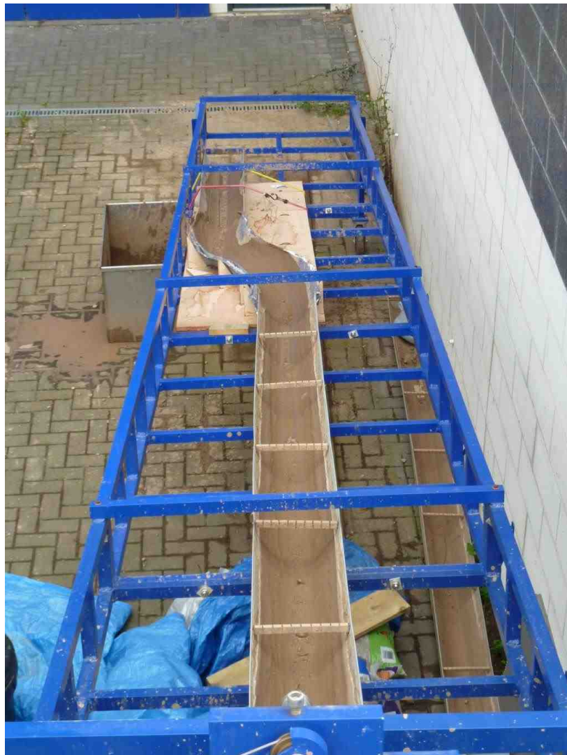
Figure 3.10: Channel bend inserted into the flume structure. The geometry of the channel bend is R_c = 0.7 \text{ m} , \theta = 40^\circ
