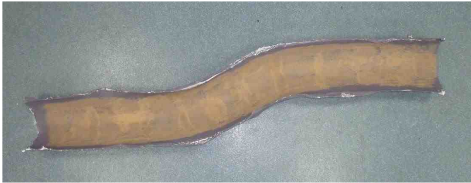
Figure 3.9: A completed bend having been reinforced, painted and a sand coating applied. Bend is R_c = 0.55 \text{ m} , \theta = 40^\circ
