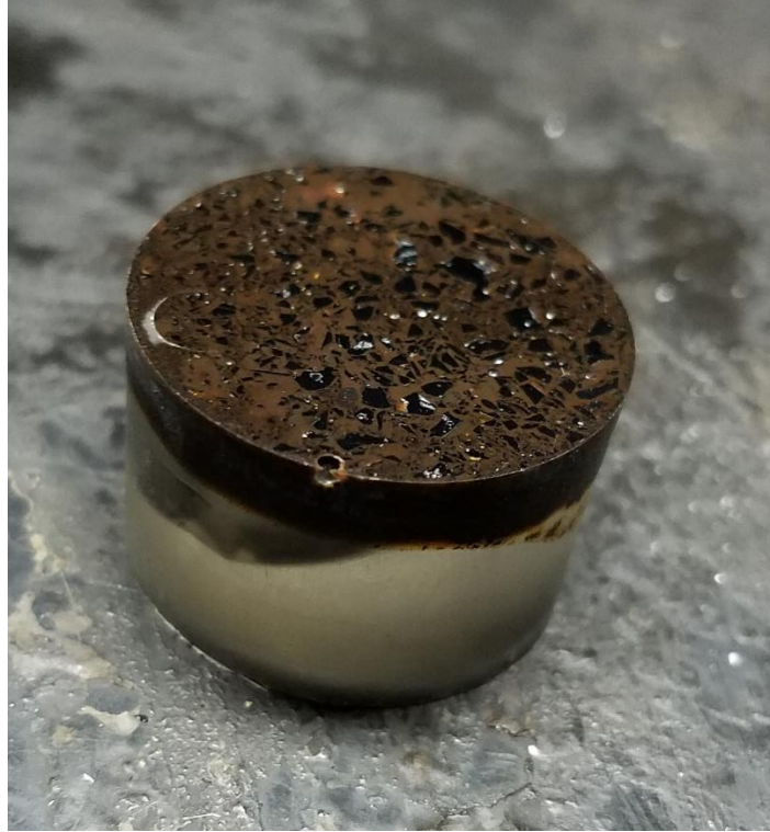
Figure 2.5 Example of a polished “puck” of pitch inside an epoxy. This “puck” was used for polarized light microscopy to determine the mesophase percentage of the heat-treated pitch. Puck was 1 inch in diameter.
