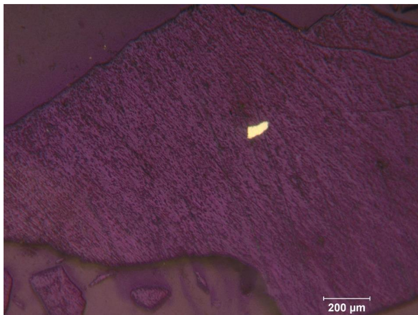
Figure 2.17 Isotropic coal-based pitch under polarized light. No mesophase content is present. The white dot is epoxy.
