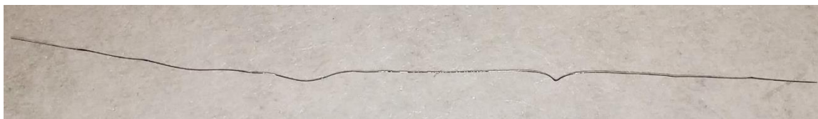
Figure 4.2 Example of a fiber that had non-uniform shrinkage during thermal conversion. Here the fiber was approximately 120 mm in length and approximately 30 \mu\text{m} in diameter.
