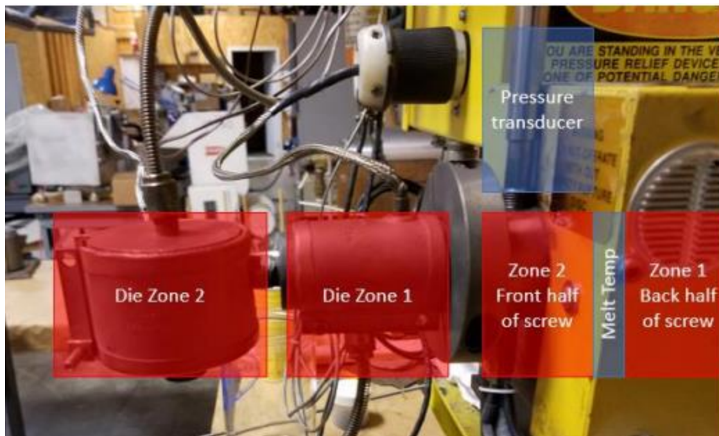
Figure 3.4 Controlled temperatures zones for the WEXT where the pitch transitions from right to left. Melt temperature and pressure transducer location are shown.
