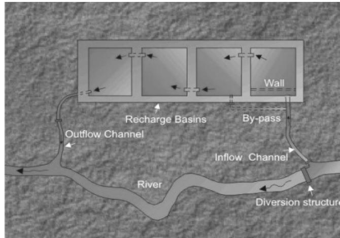
**Figure (2.1): Infiltration basins (Jemal, 2006)**
