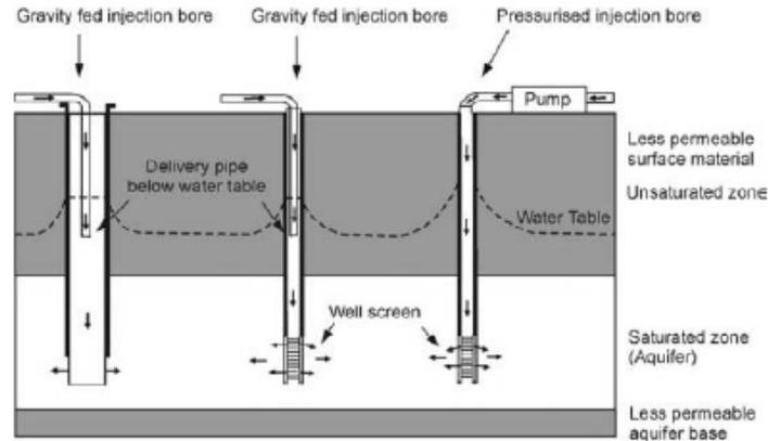
**Figure ( 2.2): Gravity injection wells or bore (Jemal, 2006)**
