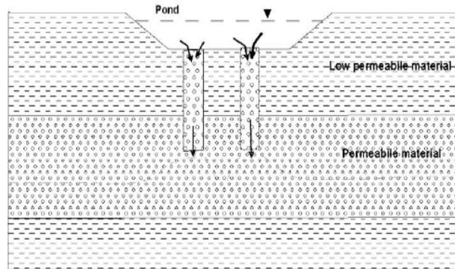
**Figure (2.3): Combination of injection well and basin (Jemal, 2006)**
