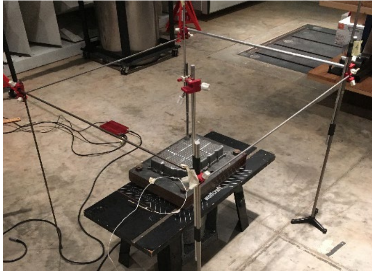
Figure 3.18 – Imaginary box constructed around the oil pan for sound intensity scan. Imaginary surfaces are 30 cm from each face of the pan.
