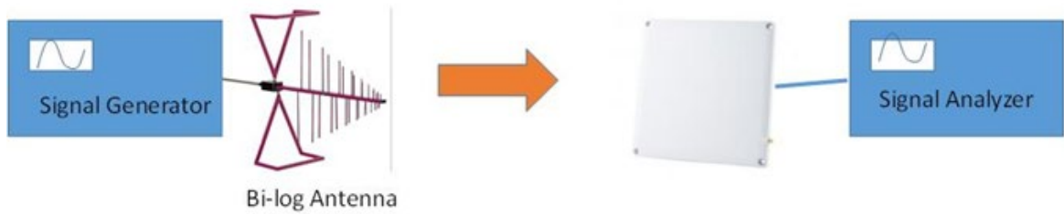
Figure 12-2: Test set up to check the error in the circularly polarizing antenna
