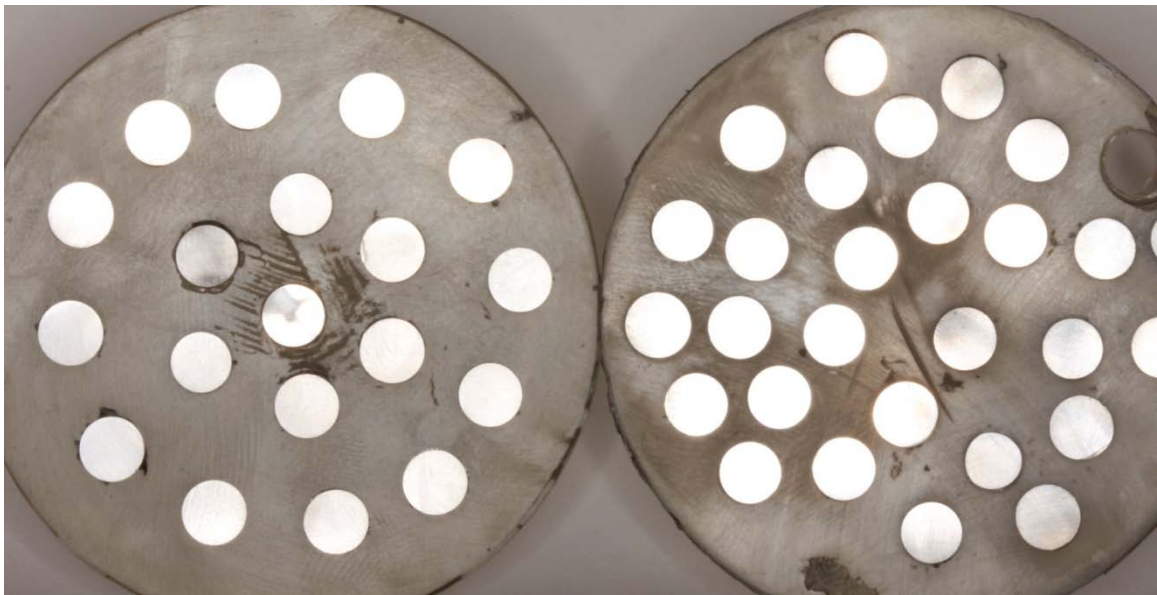
Figure 1. Samples after grinding with 600 grit silicon-carbide paper.
