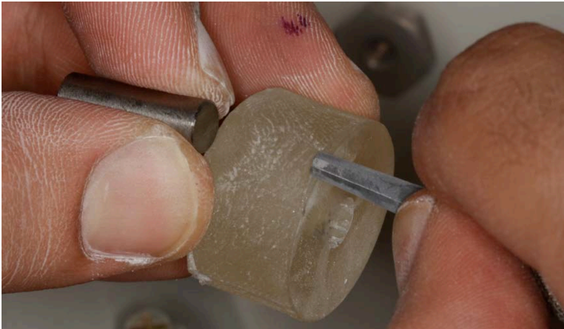
Figure 3. A specimen being sandblasted using the acrylic jig.
