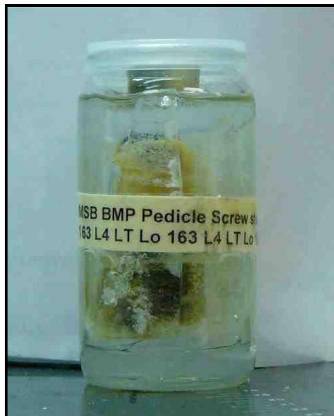
Figure 3-6. Processed specimen of the vertebral body and pedicle screw embedded in methyl methacrylate and labeled
