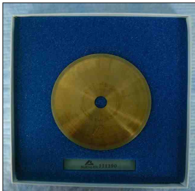
Figure 3-7. Diamond coated wafering blade used for sectioning of the vertebral body specimens
