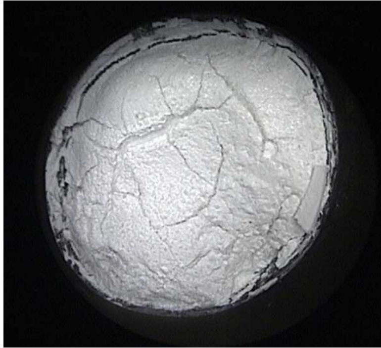
Fig; 7 ERRM exposed to EDTA (17%) for 7 days (Group II)
