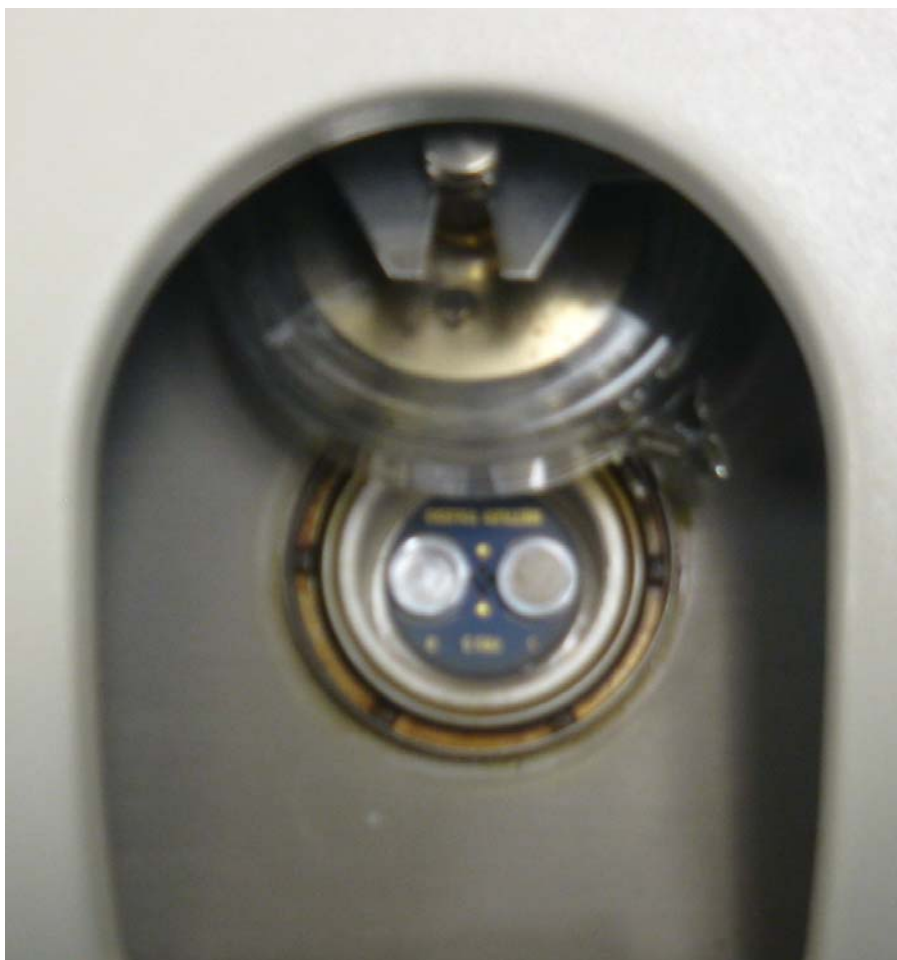
Figure 7: DSC sensor containing RMGI filled sample crucible and an empty reference crucible in their respective positions.
