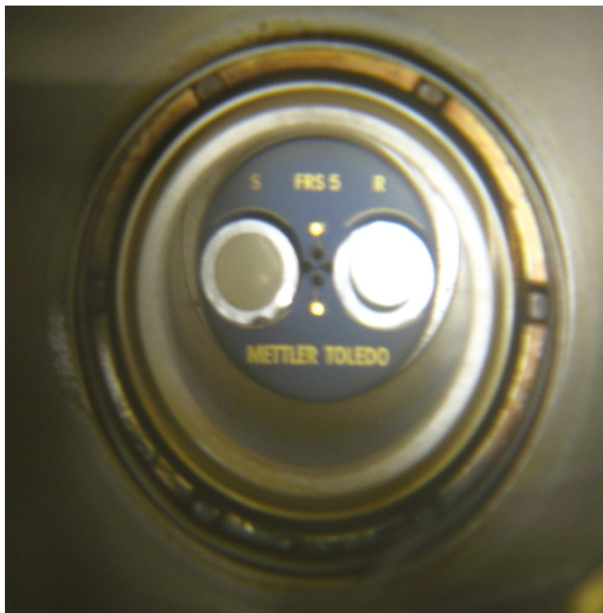
Figure 8: Close-up view of the DSC sensor containing RMGI filled sample crucible and an empty reference crucible in their respective positions.
