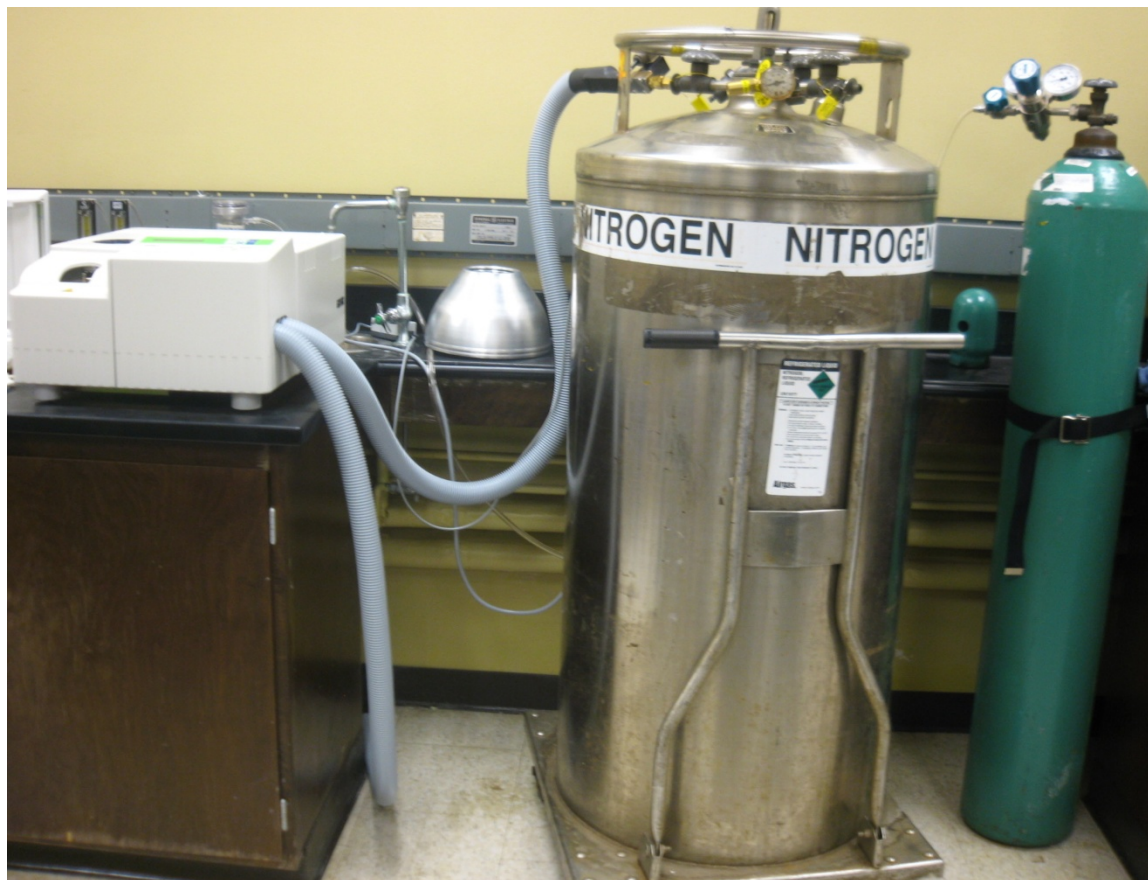
Figure 6: DSC connected to the liquid nitrogen cooling system used in the study.
