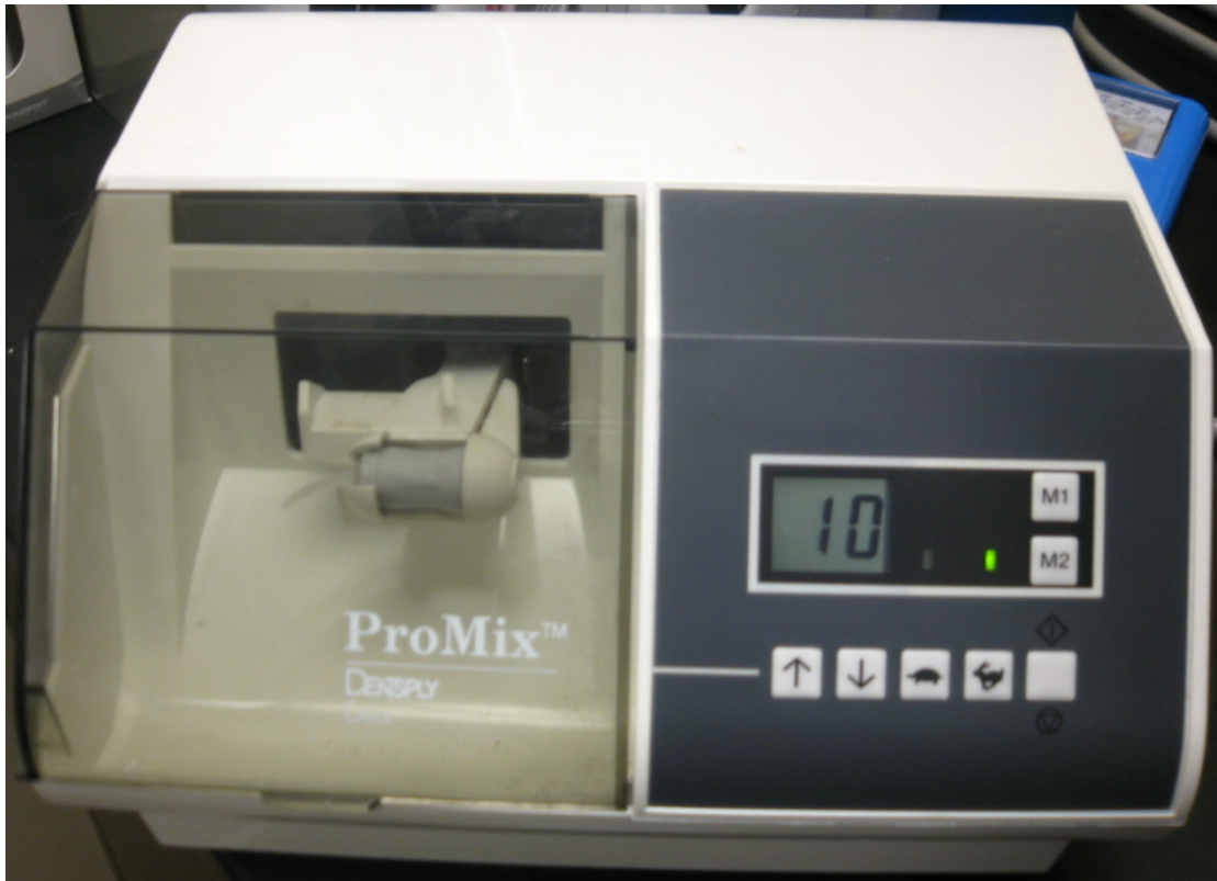
Figure 4: The amalgamator containing the activated RMGI capsule used to mix the material.
