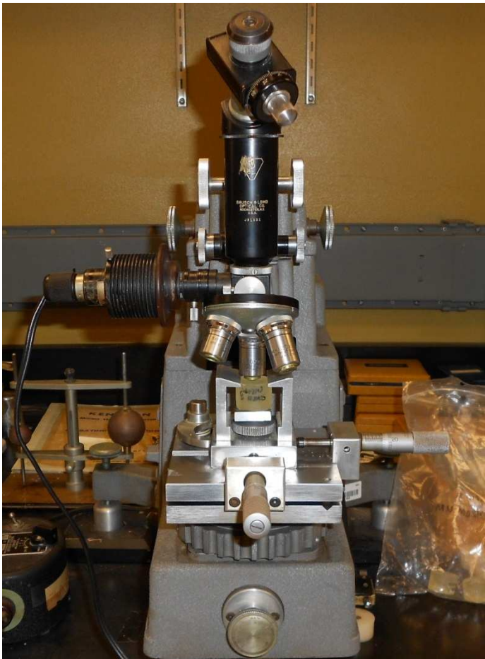
Figure 5. Kentron Vickers microhardness tester with acrylic block mounted.
