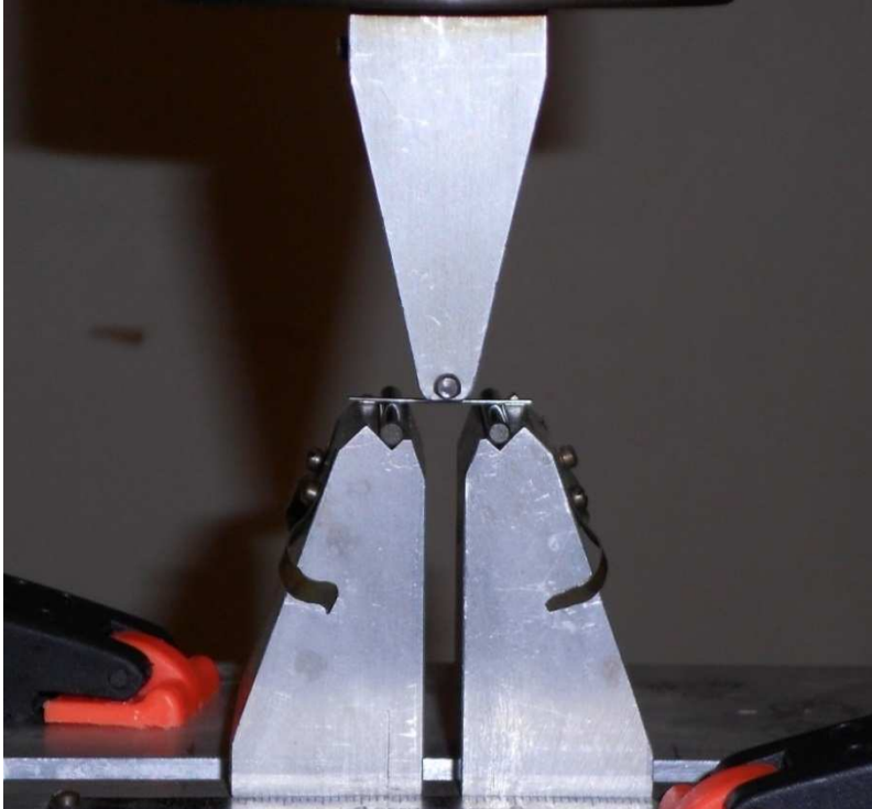
Figure 2. Testing set-up for three-point bending. A 14 mm span length between lower supports was used with the upper beam centered at 7 mm.
