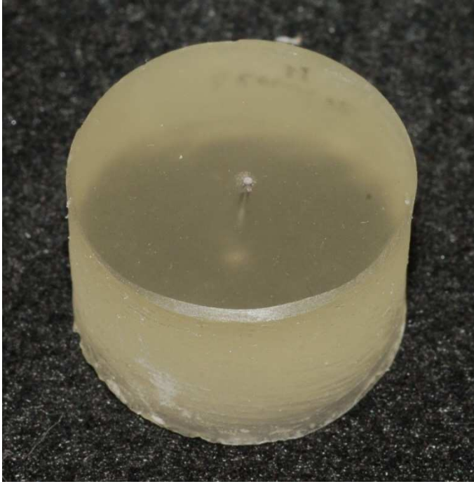
Figure 6. Polished acrylic block with wire vertically positioned for Vickers microhardness test.
