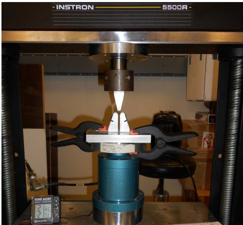
Figure 1. Instron 5500R utilized for data collection during the three-point bending test.
