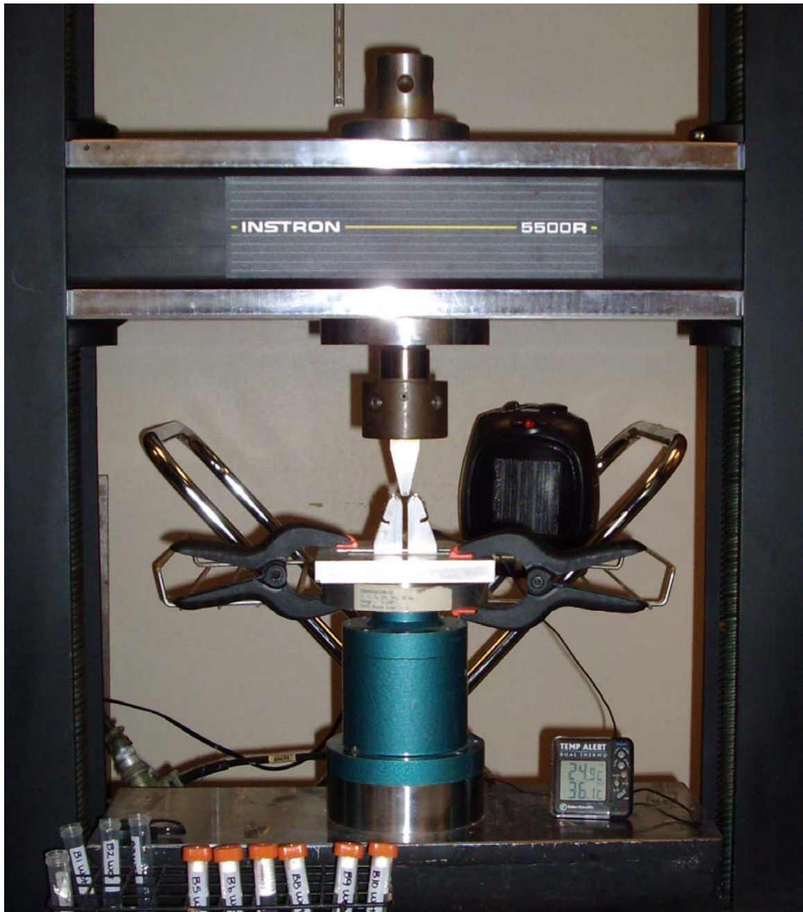
Figure 5. Instron 5500R with the testing platform. The temperature is controlled by the portable heater in the back and monitored with the probe attached to the platform.
