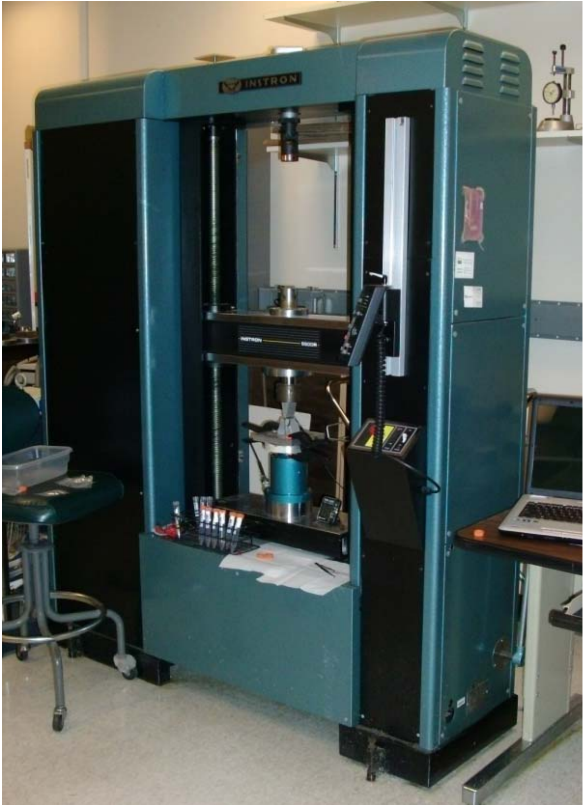
Figure 4. Instron 5500R machine for 3-point bending test.
