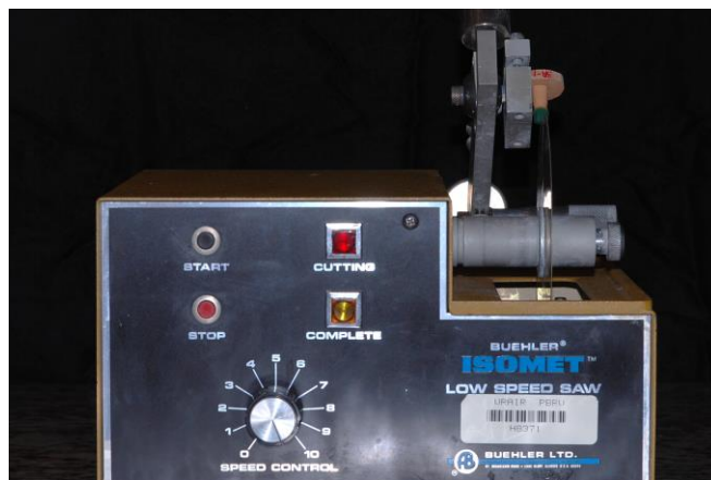
Figure 21. Sectioning of the specimen with the low speed saw
