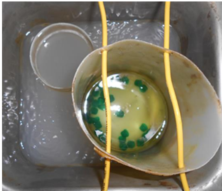
Figure 11. Ultrasonic cleansing in 100% corn oil
