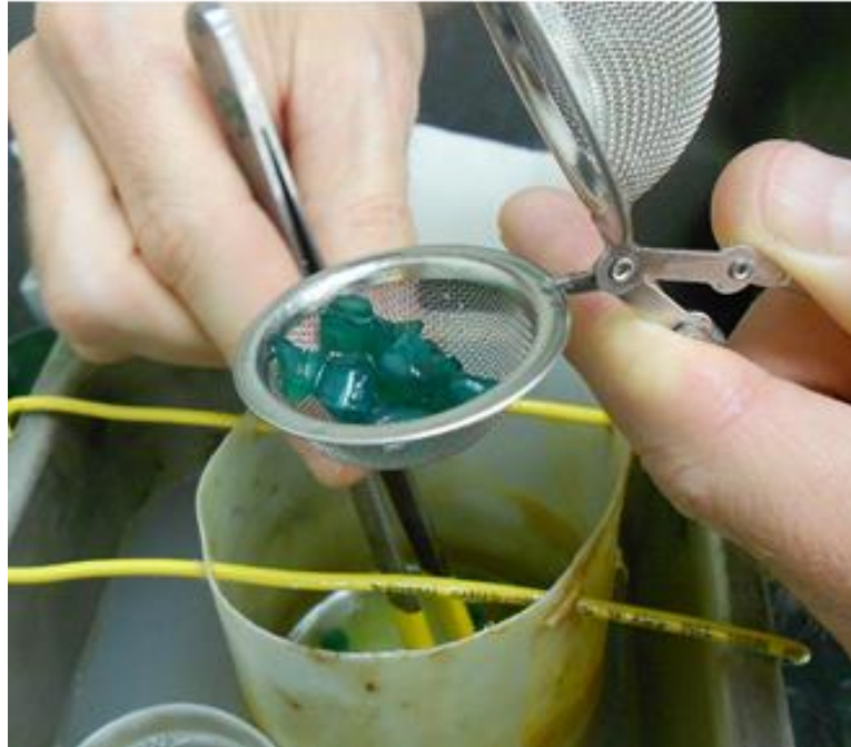
Figure 12. Removal of resin copings from the corn oil solution
