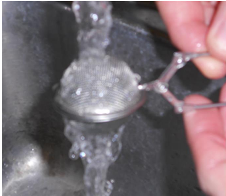
Figure 13. Removing residual corn oil from copings
