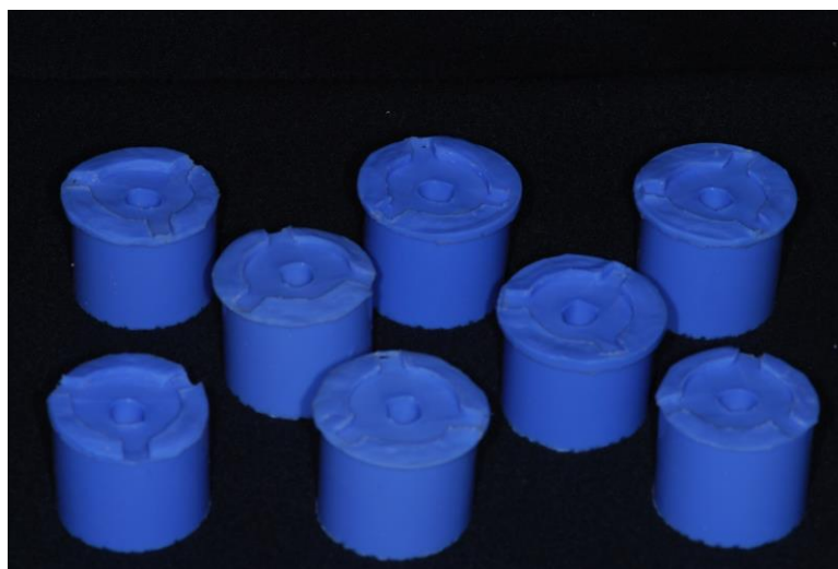
Figure 4. Duplicating silicone molds
