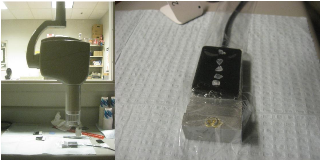
Figure 2-7: Radiographic measurement of the bone microdensity
