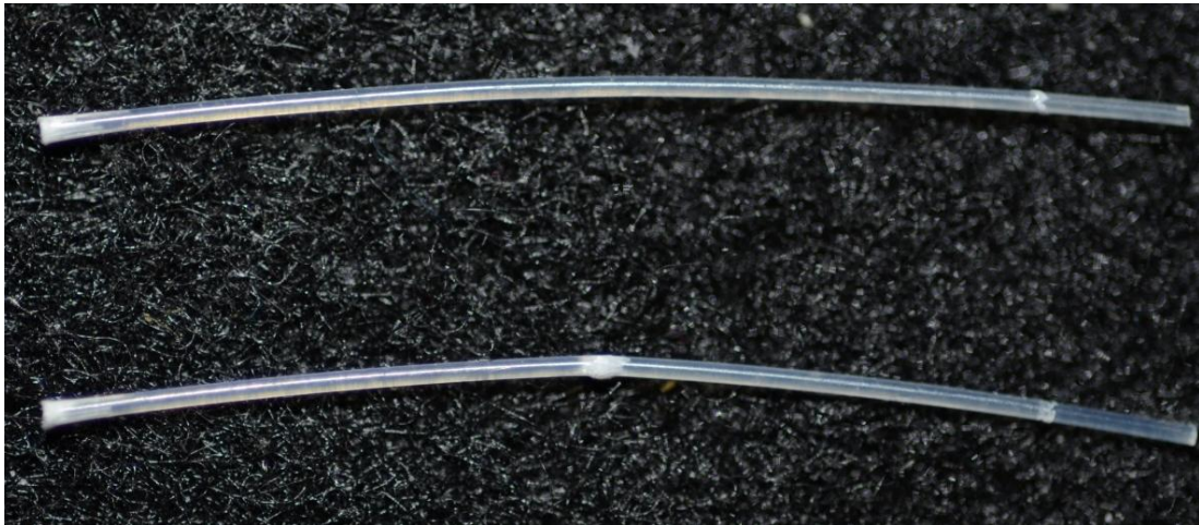
Figure 16. Comparison of non-crazed (top) and crazed (bottom) fiber-reinforced composite archwire.
