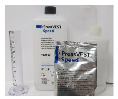
Figure 2. IPS VEST Speed phosphate-bonded investment.
