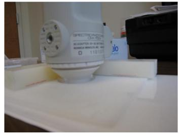
Figure 10. Spectrophotometer placement on holder.
