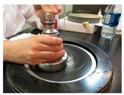
Figure 6. Grinding of specimens with silicon carbide paper to achieve 3 mm thickness after stain application.
