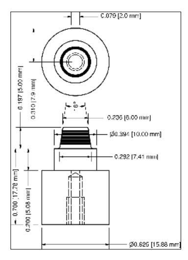
Figure 1 – Dimensions of dies
