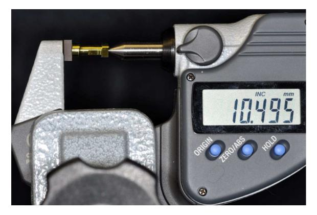
Figure 10: Measuring implant analog length.
