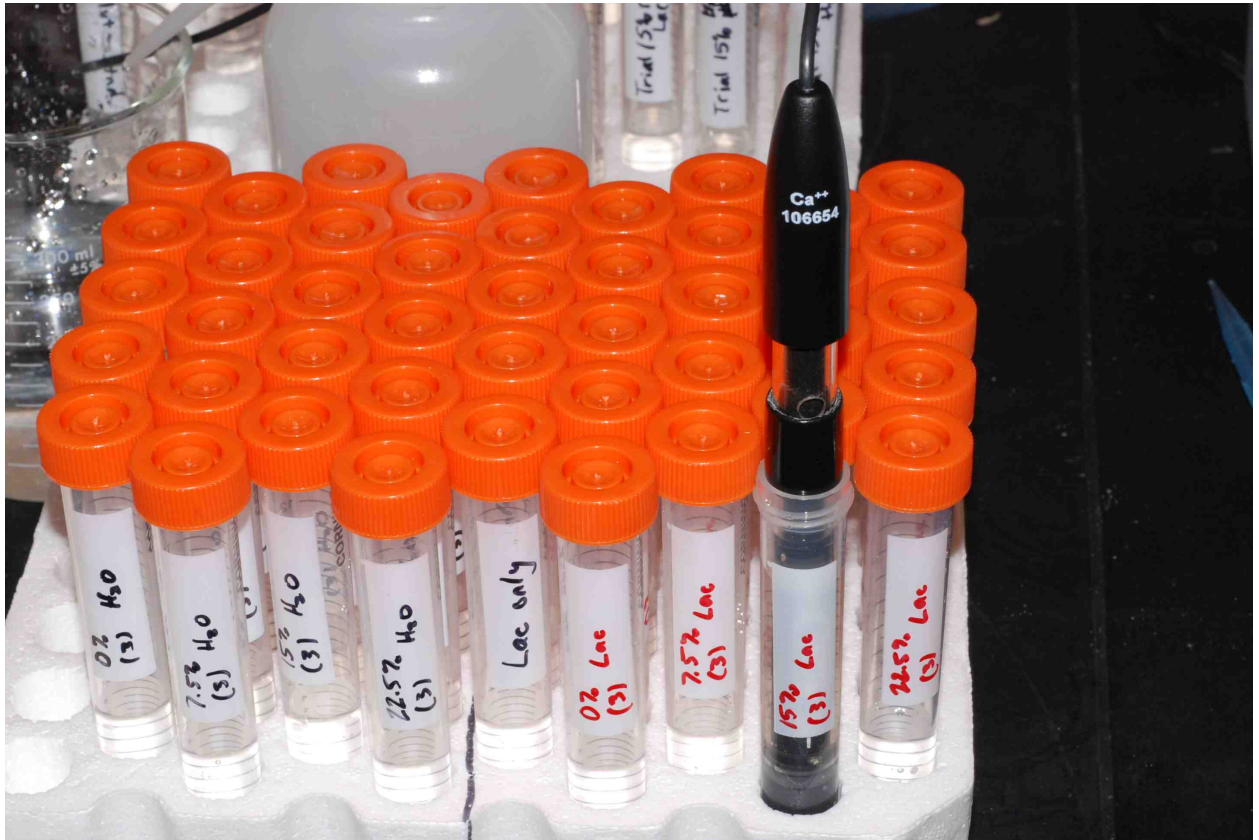
Figure 2. Specimen array and electrode measurement setup
