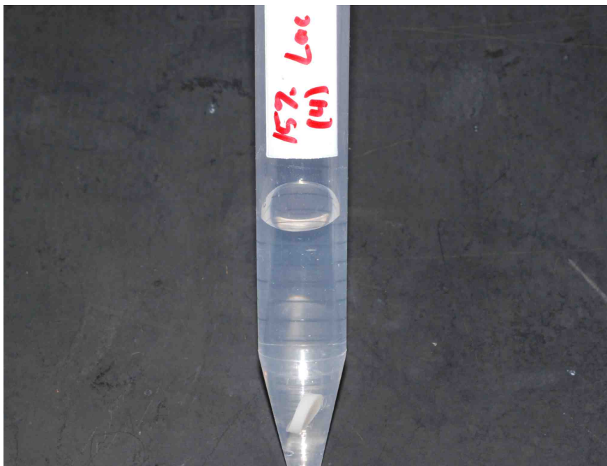
Figure 1. Resin disc immersed in 5 mL lactic acid solution.
