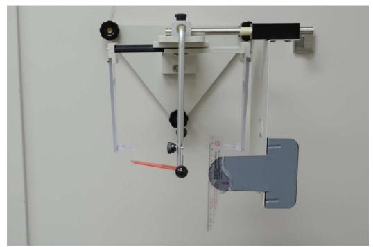
Figure 1 Head positioning apparatus
