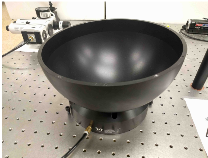
Figure 5.8: The spherical air bearing allows for three rotational degrees of freedom.
