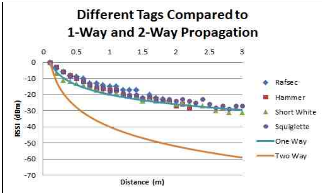
Figure 4-8 The theoretical model for one-way and two-way reflection showing the expected decrease in signal strength, compared to normalized data taken for RFID tags tested in an anechoic chamber.
