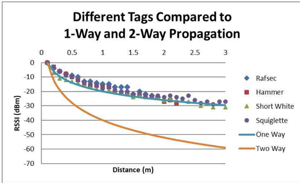
Figure A-9: Data collected on RSSI as a function of distance follows a one-way propagation model. (Figure 4-9 reproduced)
