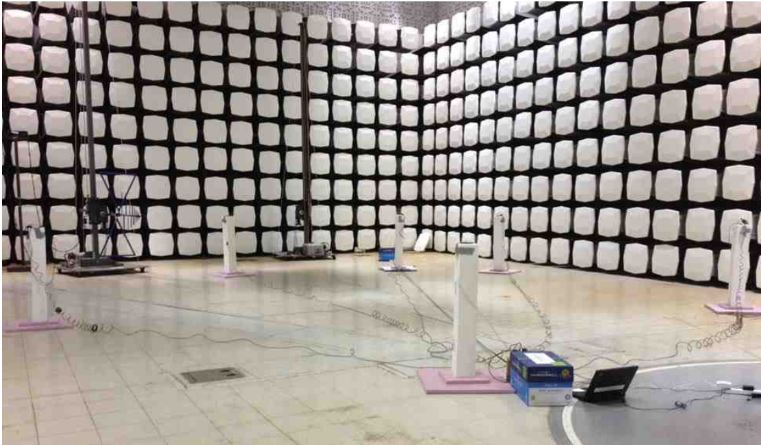
Figure 11-3: BLE localization data collection in 10 meter anechoic chamber.
