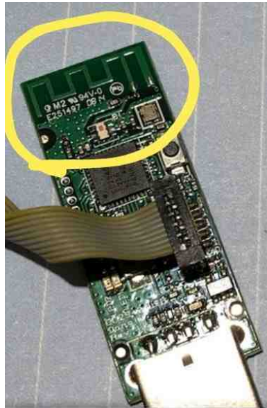
Figure 3-2: BLE device used for this work, highlighting the imbedded antenna.
