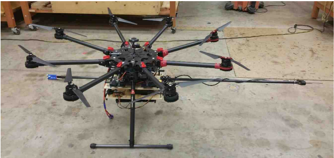
Figure 4.4: BLUECAT 4 multi-rotor equipped with hot-wire instrumentation.
