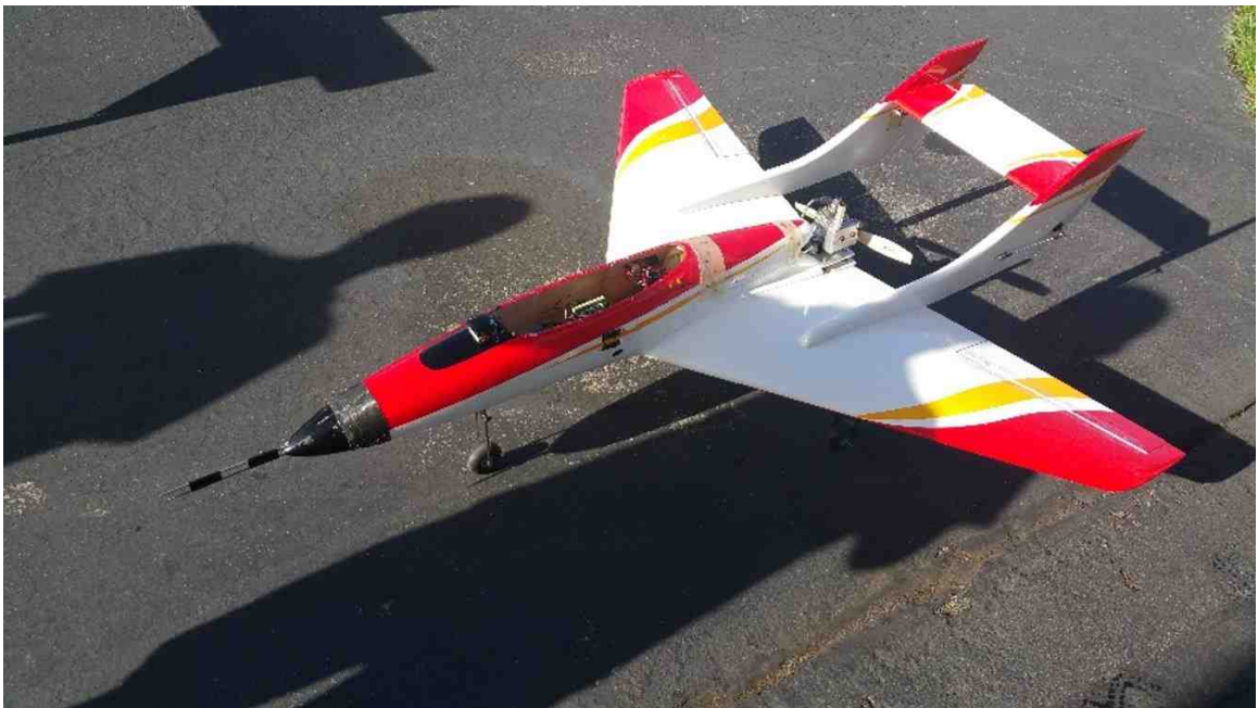
Figure 4.3: BLUECAT 3 airframe equipped with hot-wire instrumentation.
