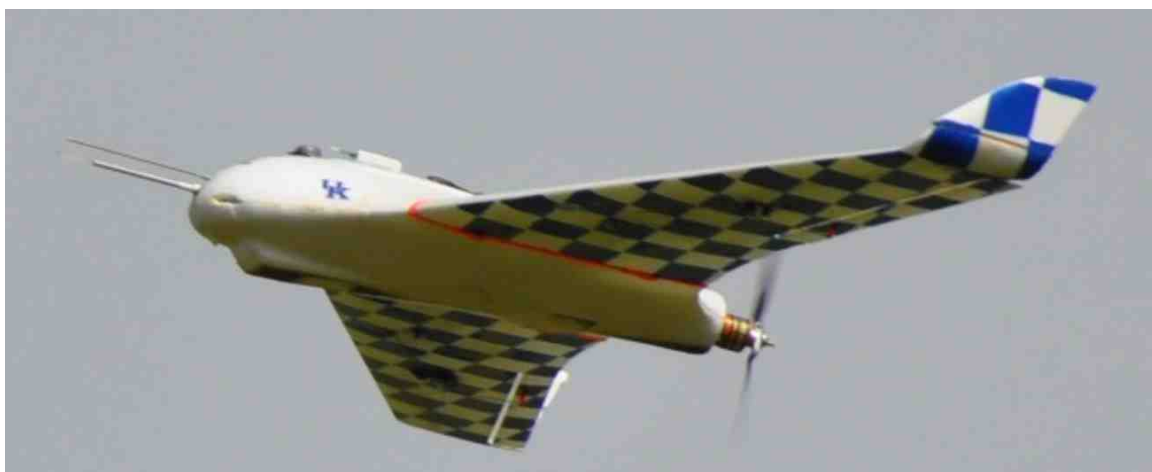
Figure 4.5: BLUECAT 5 equipped with five hole probe instrumentation.
