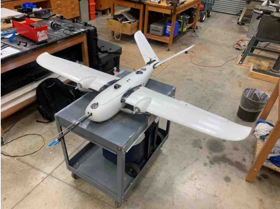
Figure 5.1: BLUECAT 6B outfitted with hot-wire anemometer and five hole probe sensors.
