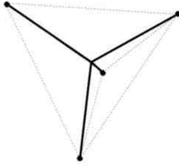
Figure 1.14: Four weighting vectors for 3D balanced multi-point encoding method
