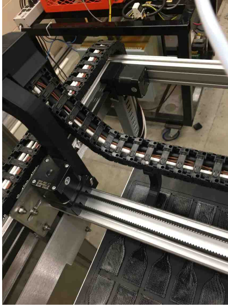
Figure 1.6: FFD printer “X” and “Y” travel mechanism
