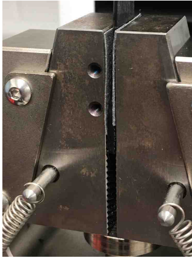
Figure 3.16: Specimen install using 240-grit sandpaper to prevent slipping at high strains
