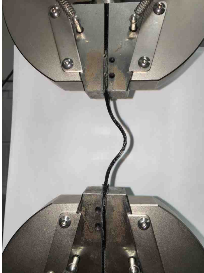
Figure 3.36: Specimen folding at Instron initial position, indicating permanent deformation
