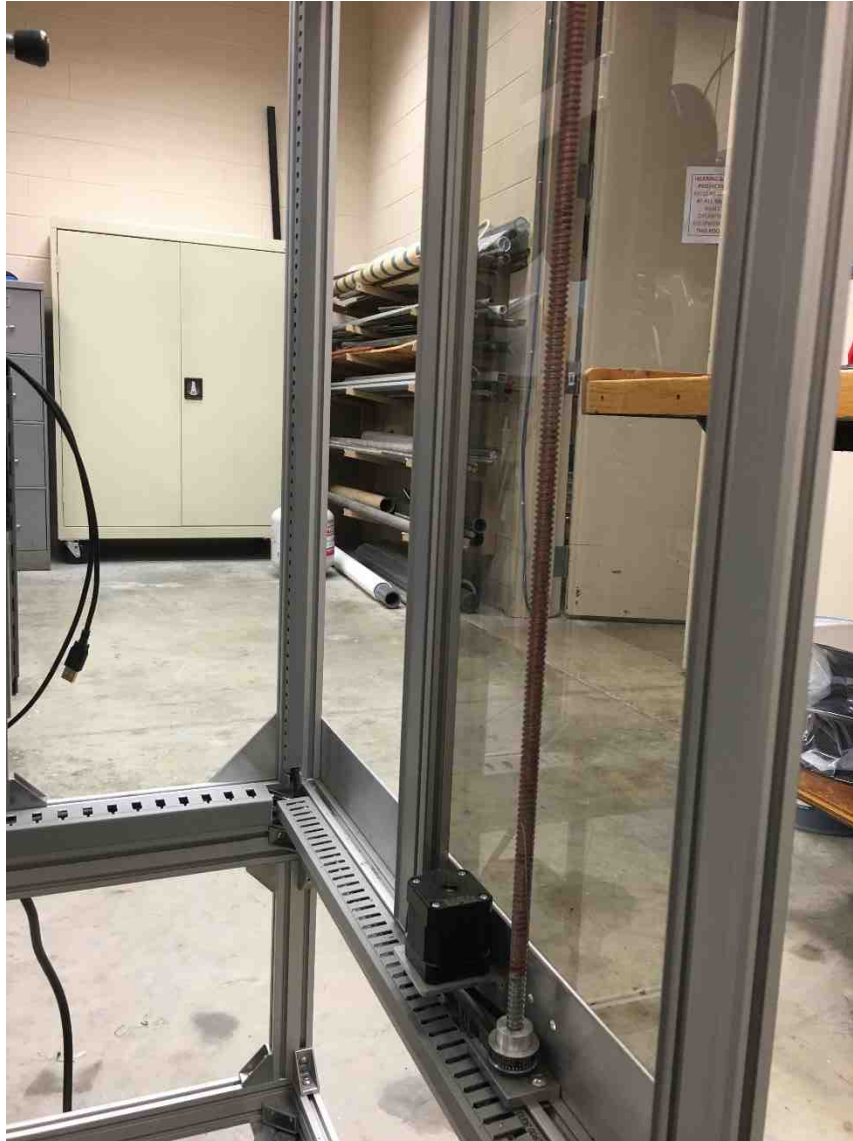
Figure 1.7: FFD printer "Z" travel mechanism
