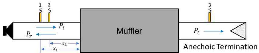
Figure 2.8 Transmission loss measurement with the three-point method
