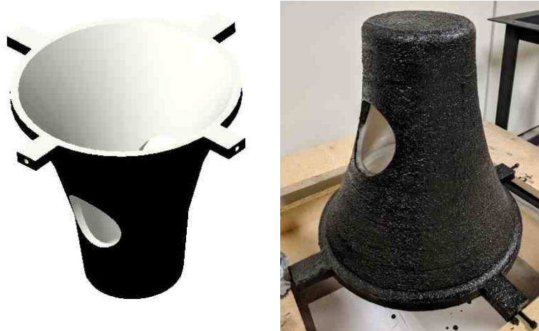
Figure 3.9 Inverted exponential horn
