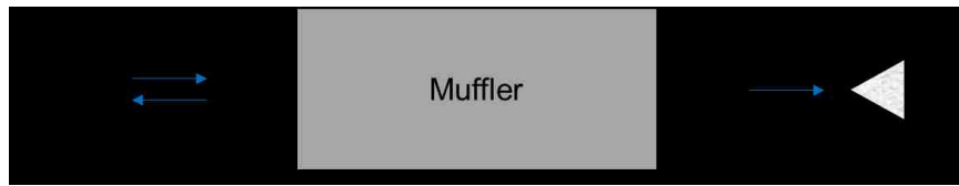
Figure 2.7 Transmission loss definition sans flow [16]
