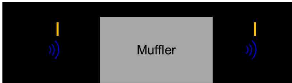
Figure 2.11 Noise reduction measurement setup
