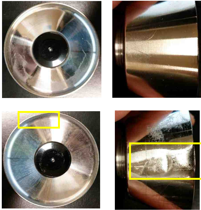
Figure 3.2. Undamaged cup from (top left) front and (top right) side view along with damaged cup from (bottom left) front and (bottom right) side view for comparison.
