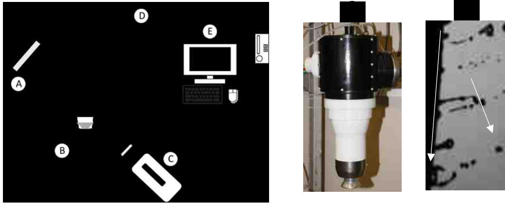
Figure 1.2. Experimental diagram (left) with lamp (A), rotary bell (B), camera (C), hood (D) and computer (E). Also pictured are the rotary bell (F) and an experimental image (G) with direction of cup rotation (left arrow) and the general fluid flow direction (right arrow) indicated.
