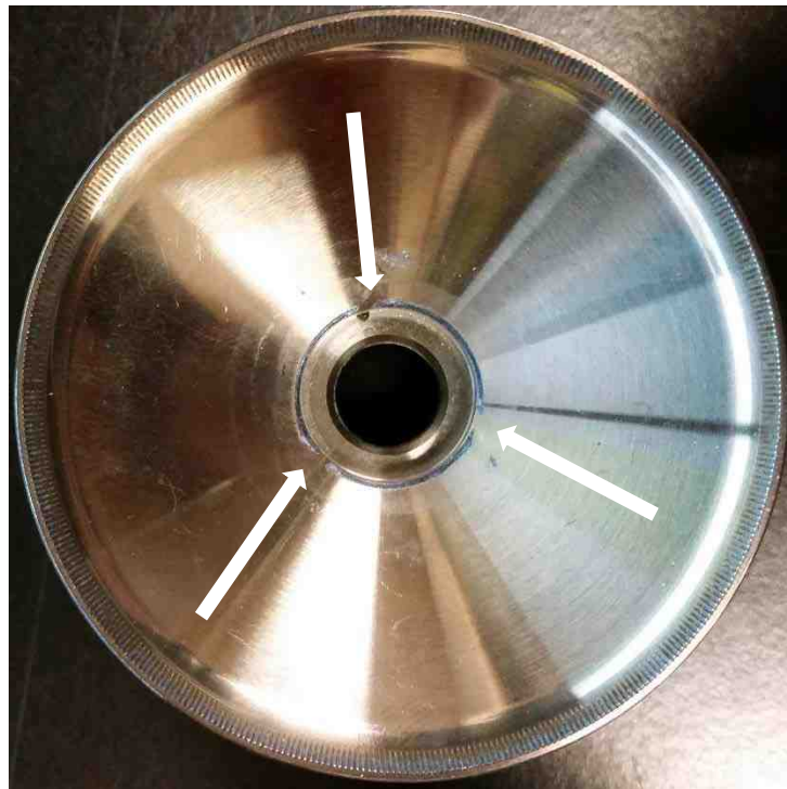
Figure 3.11. Rotary bell with center cap removed to display fluid outlets (indicated by arrows) to the interior of the bell, through the glue residue of the cap.
