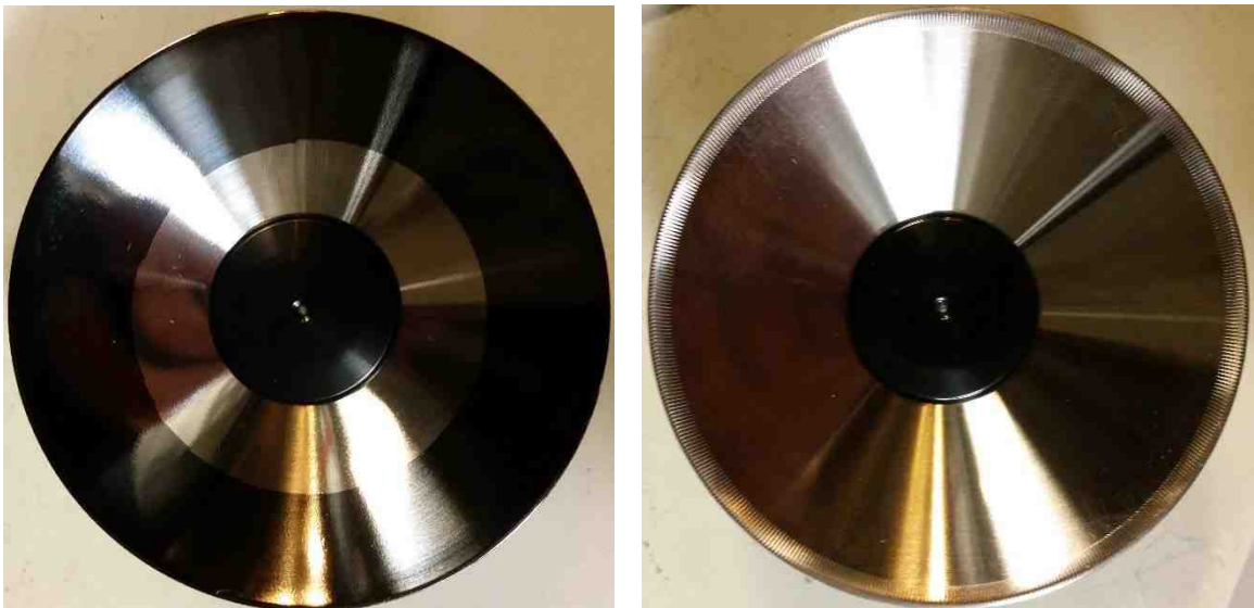
Figure 2.1. Unserrated (left) and serrated (right) 65mm bell-cups.
