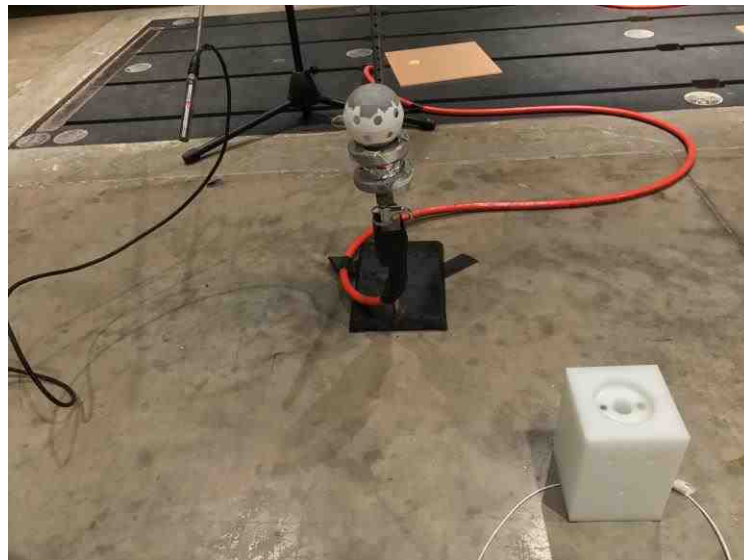
Figure 6.2 Transfer function measurement setup for full model
