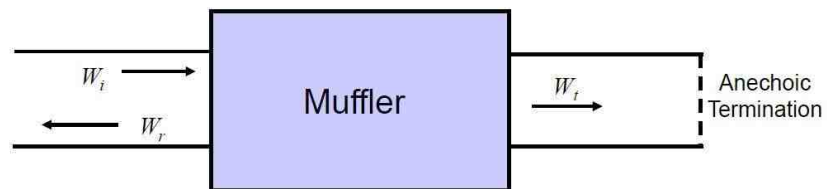
Figure 2.6 Definition of muffler transmission loss
