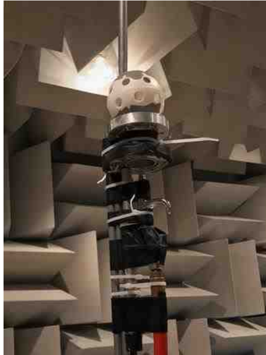
Figure 2.4 Point source at University of Kentucky Vibro-Acoustic Lab
