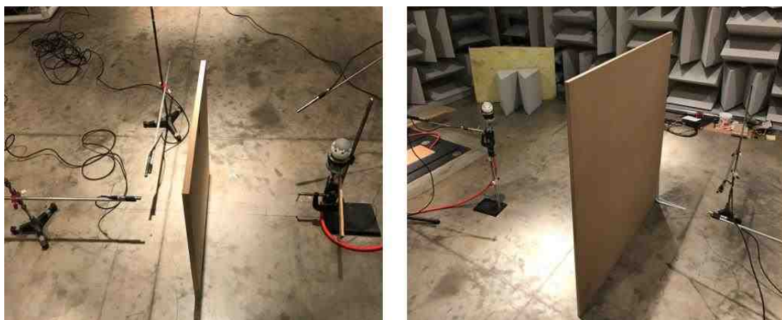
Figure 4.3 Measurement setup for full barrier and its scale model
