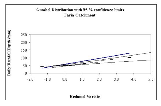
**Figure 24:** 95% Confidence Limits of Upper Faria catchment-Gumbel Distribution
