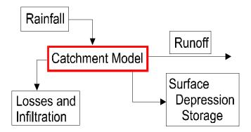
Figure 6: Rainfall-runoff modeling using surface water budget
