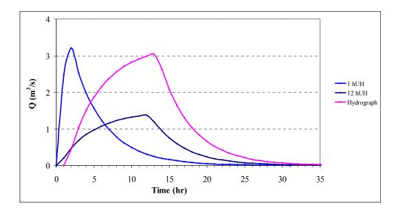
Figure 33: Routing of the Upper Faria Unit Hydrograph
