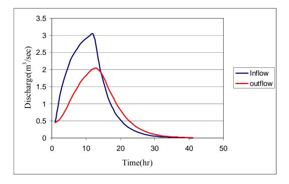
Figure 34: Routing of the Inflow Hydrograph into the Storage Reservoir.
