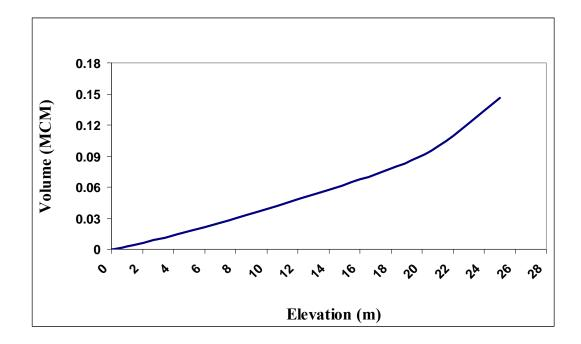
Figure 31: Elevation and Storage Volume of the Proposed Dam
