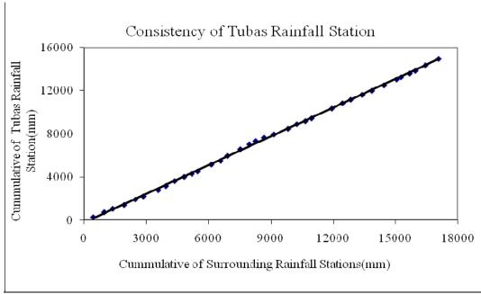
Figure 12: Double Mass Analysis for Tubas Station, (1967-2003)
