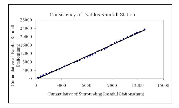
Figure 15: Double Mass Analysis for Nablus Station, (1967-2003)
