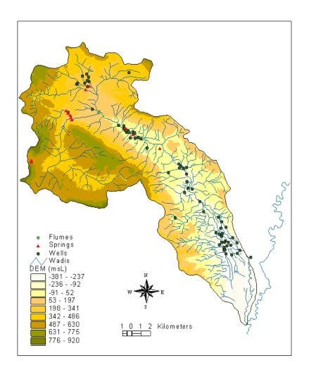
Figure 3: Topography and Stream System of Faria catchment.
