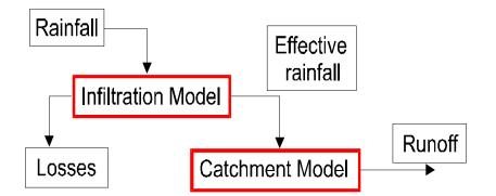
Figure 5: Rainfall-runoff modeling using effective rainfall
