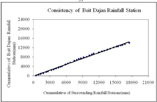
Figure 16: Double Mass Analysis for Beit Dajan Station, (1967-2003)
