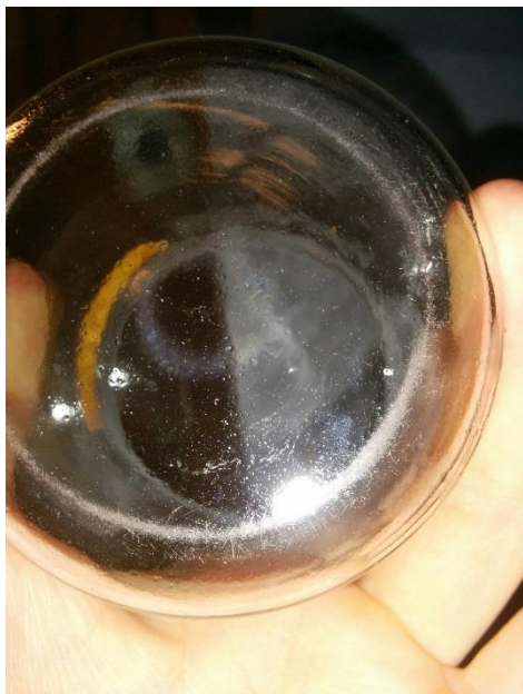
Figure 27. Calcareous fur residue after evaporating 50 % of the sample amount.
