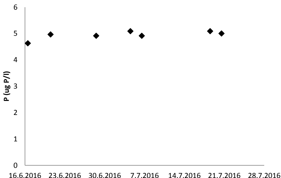
Figure 28. 5 \mu\text{g P/l} follow up of known phosphorus concentration (SFS EN ISO 6878 with 10 cm cuvette).
