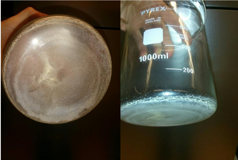
Figure 26. Calcareous fur residue after evaporating water samples completely.
