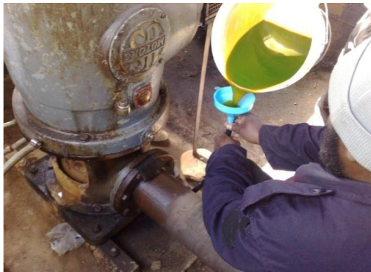
a) Slug injection of Uranine tracer into a well injection
