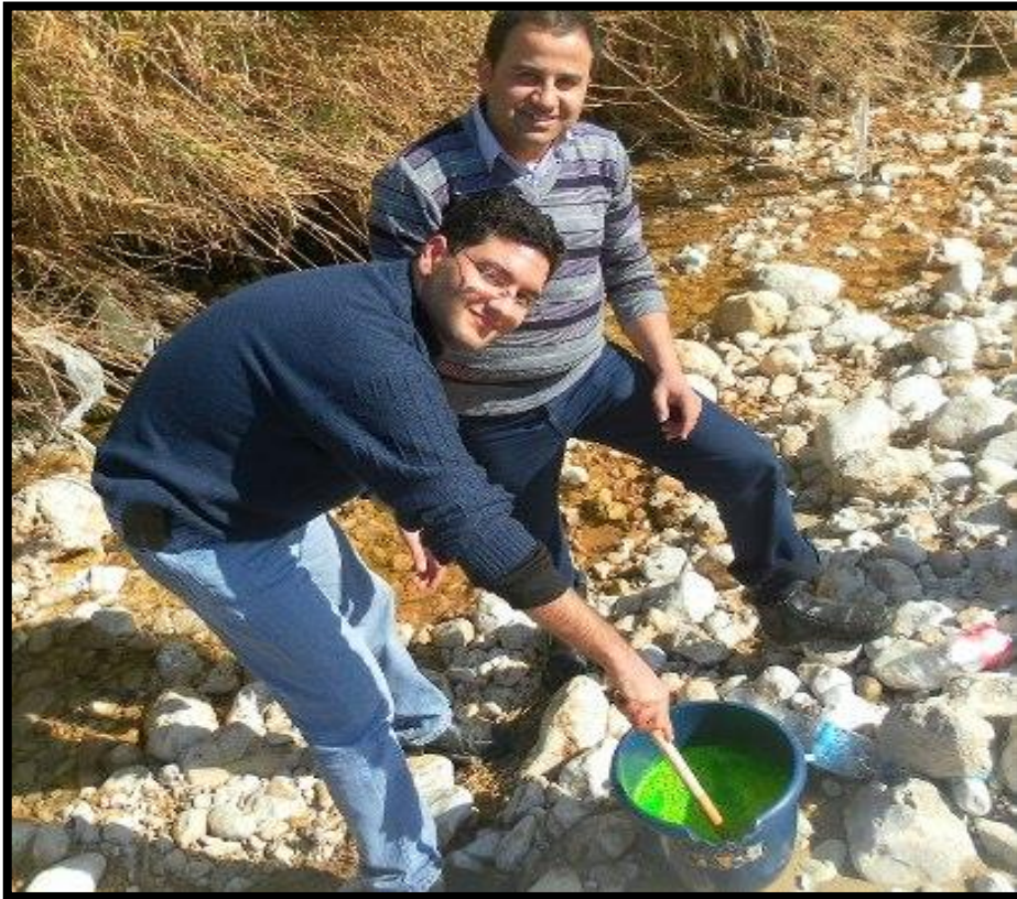
Figure 42: Dissolving and mixing of Uranine solution
