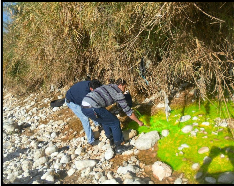
Figure 43: Pouring of Uranine solution into the wadi
