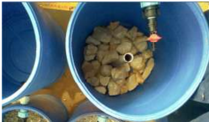
Figure (3-4): The first layer in the constructed wetland consisted of gravel for a 13cm-depth.
