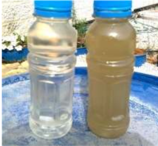
Figure (4-31): Photo showing the wastewater before (right) and after (left) treatment process.
