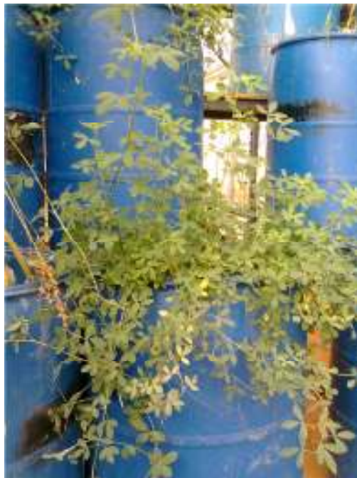
Figure(4-17): The plant grows and spreads in both directions Vertical and Horizontal so the aeration from the atmosphere to the system was less, DO =2.5 mg/l
