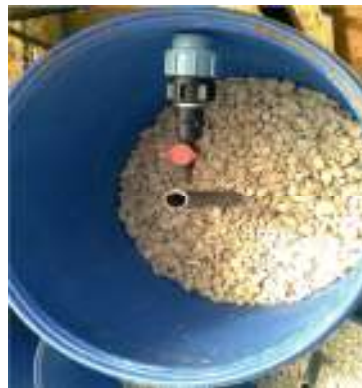
Figure (3-5): Constructed wetland with total height for media equal to 50 cm.
