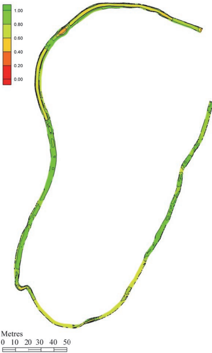
Fig. 7. Summer rearing habitat suitability for juvenile salmon with >10 cm body length at 1.0 m 3 /s discharge in the entirely natural-like bypass at the Montta hydropower plant in the river Oulujoki.
