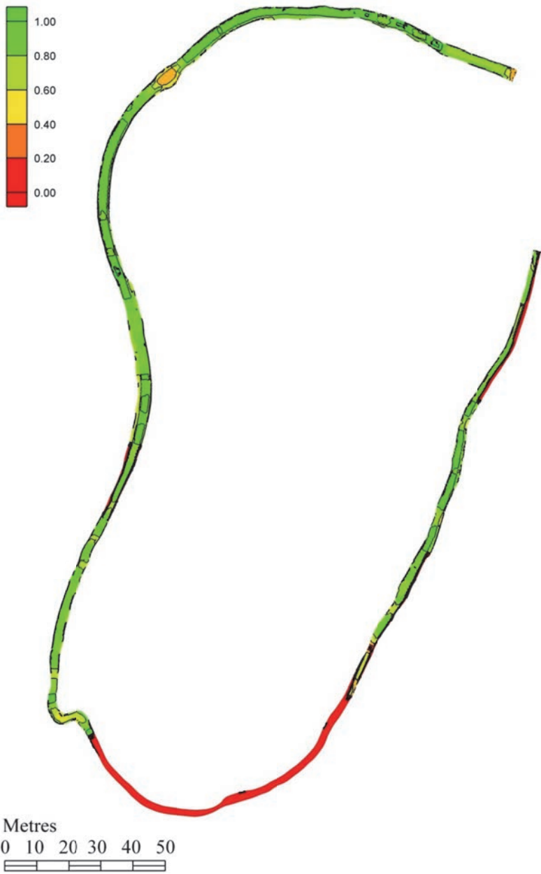
Fig. 5. Spawning habitat suitability for salmon at 0.5 m 3 /s discharge in the entirely natural-like bypass at the Montta hydropower plant in the river Oulujoki.
