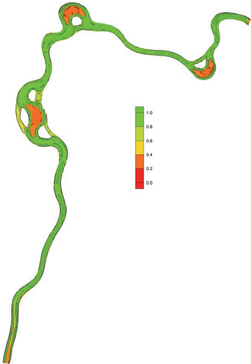
Fig. 11. Juvenile habitat suitability for salmon at 0.8 m 3 /s discharge in the upper natural-like section of the new design bypass at the Montta hydropower plant in the river Oulujoki. Suitability value calculated assuming bottom material habitat value to be 1.
