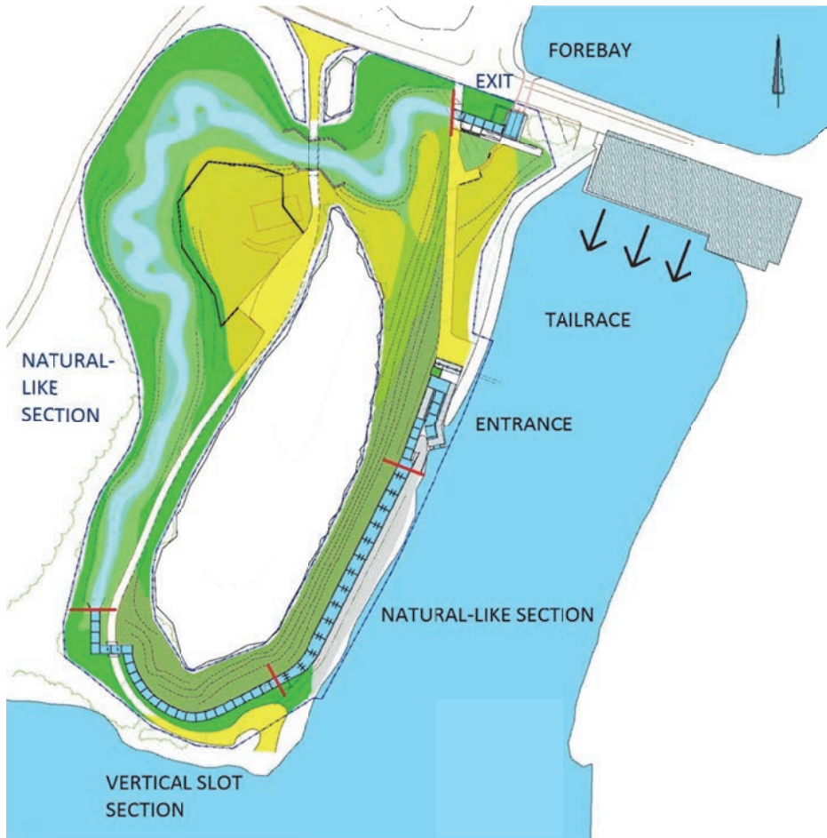
Fig. 9. The new design of the Montta bypass. The bypass consists of three vertical slot sections and two natural-like sections. Section change areas are marked in the diagram with red lines. Diagram prepared by VSU Arkkitehtuuri- ja viheraluesuunnittelu Oy.
