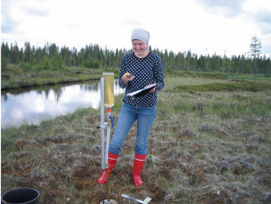
Fig. 8. Measuring hydraulic conductivity with a piezometer (photo by A.-K. Ronkanen).
