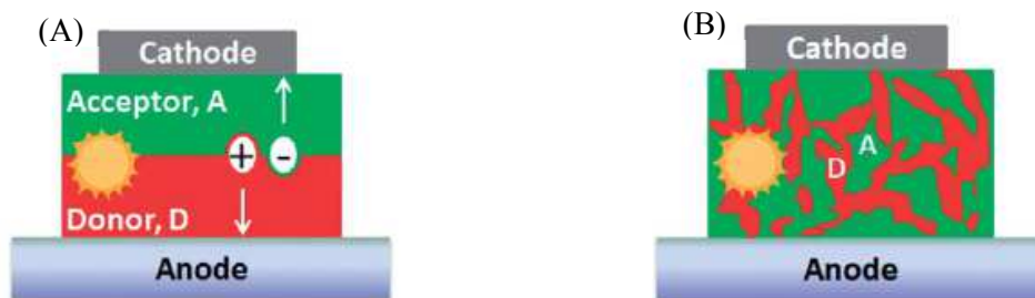
Figure 1.1 Simplified illustrations (A) bilayer structure of organic solar cells where electron acceptors are atop the electron donors; (B) bulk-heterojunction (BHJ) morphology in which the electron donors and electron acceptors are mixed intimately as the active layer. Adapted the copyright of Ref. 18 Copyright (2014), The Royal Society of Chemistry.
