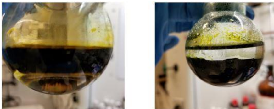
Figure 3.4 Example of the two solvent exchange method using sodium bromocresol dye where the sodium is being exchanged with TBA. Left is before exchange where the dye is in the DMSO layer and right is after exchange where the dye migrated to the chloroform layer
