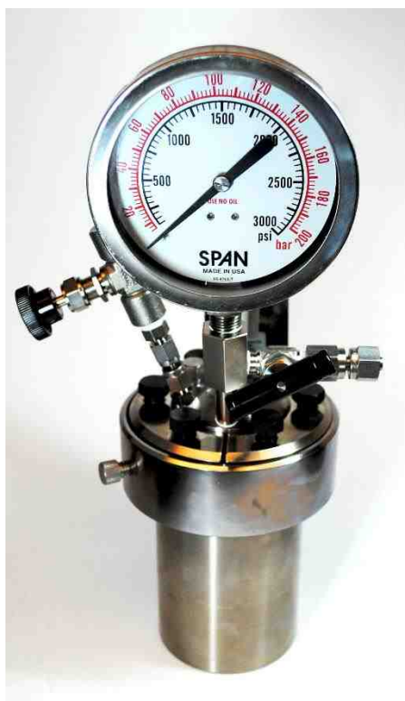
Figure 7.3 Picture of the Parr 300 mL non-stirred pressure vessel (model 4760) used in these reactions. This general-purpose pressure vessel has a maximum temperature of 350°C and a maximum pressure of 3000 psi (200 bar).
