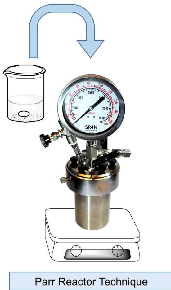
Figure 5.16 Schematic of the Parr reactor reduction set up. This set up involves a hot plate with a bored-out aluminum block which heats the reactor, producing even heating with improved heat transfer.
