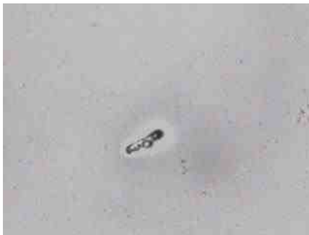
Figure 4.4. Optical image of one of typical PCBM crystal and halo ring around it
