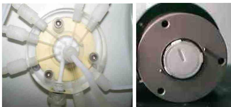
Figure 3.7 a) Left: Example of a LOV piece. b) Right: Rotor of the SV.
