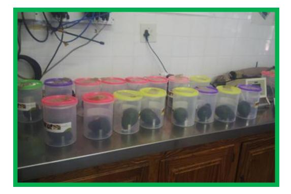
Figure 3.5 Measuring the respiration of the new 'Fuerte-type' avocado fruit
