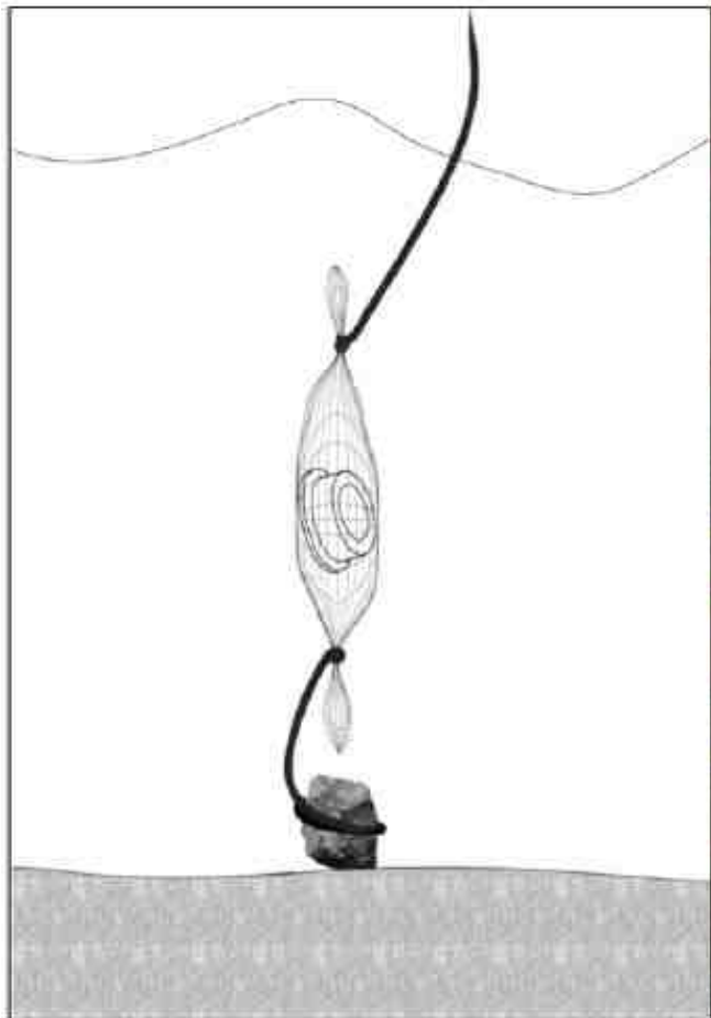
Figure 27: Illustration on how DGTs were deployed in the field (Mohr 2010) (Mohr 2012)
