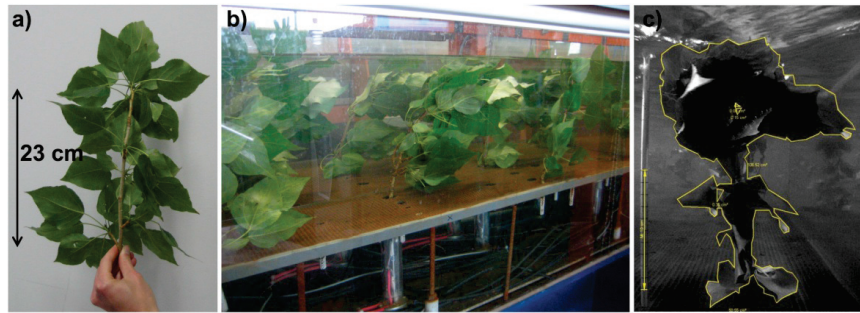
Figure 6. Representative specimen of Populus nigra (Black Poplar) (a), a P. nigra plant stand under flow (b), and determination of the frontal projected area under flow (c). (Paper II)
