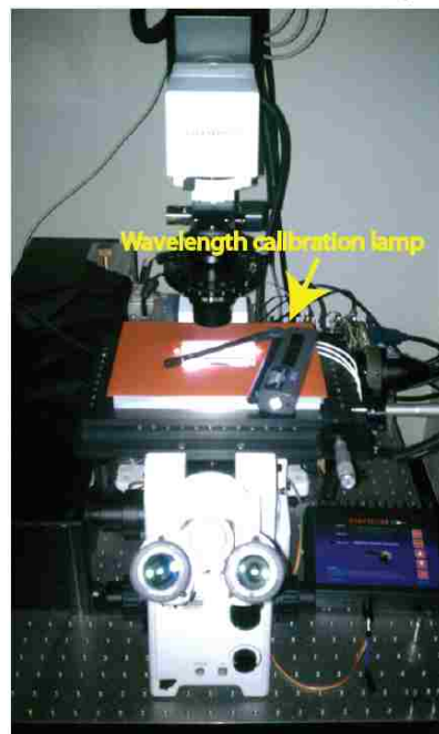
Wavelength calibration lamp positioning
