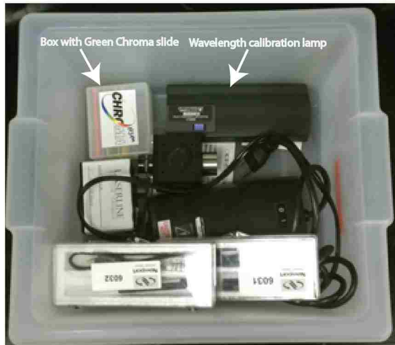
HSM Calibration box contains all components necessary for calibration.
